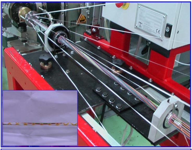
Line for lay-up in S-Z of micro cables composed of optical fibres with tight insulation or traditional conductors. Possibility to laying up in simple or double crown up to a max of 24 elements in one step.
